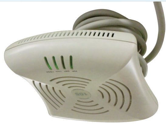
an Access Point on the ceiling to provide fast Wi-Fi network connection
